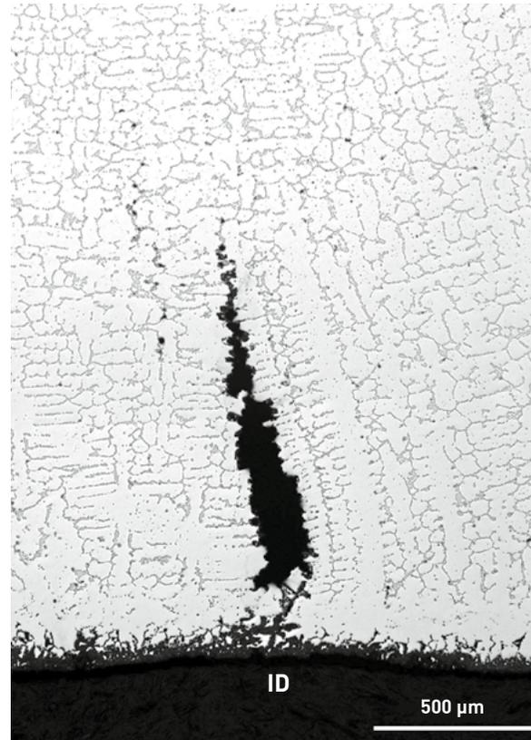
Figure 7: Higher magnification photomicrograph of creep fissure
