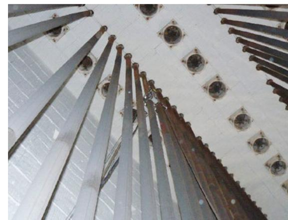
Reformer tube testing with LEO-Scan
