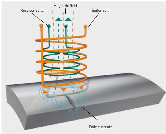
Figure 6: The principle behind eddy current testing
